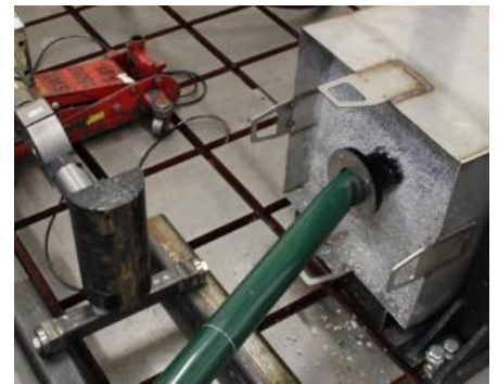
Figure 9 – Impact Loading Atlas Socket
