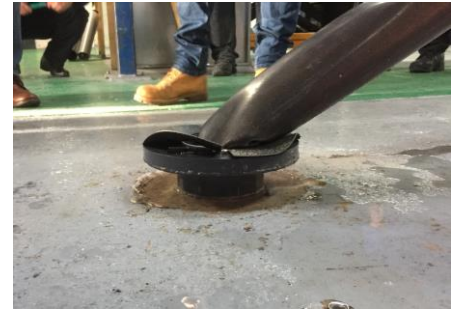
Figure 8 – Crash Testing the Atlas Socket
