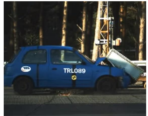
Figure 4 - Passively Safe Cabinet Crash Test
